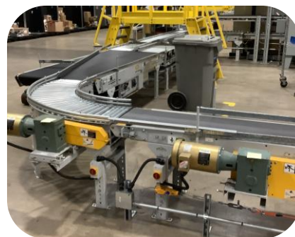
Standard 1 hp IE4 motors (gold) paired with 20:1 gearboxes (green)
