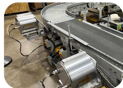
C-Motive Electrostatic machines connected via chain drives
